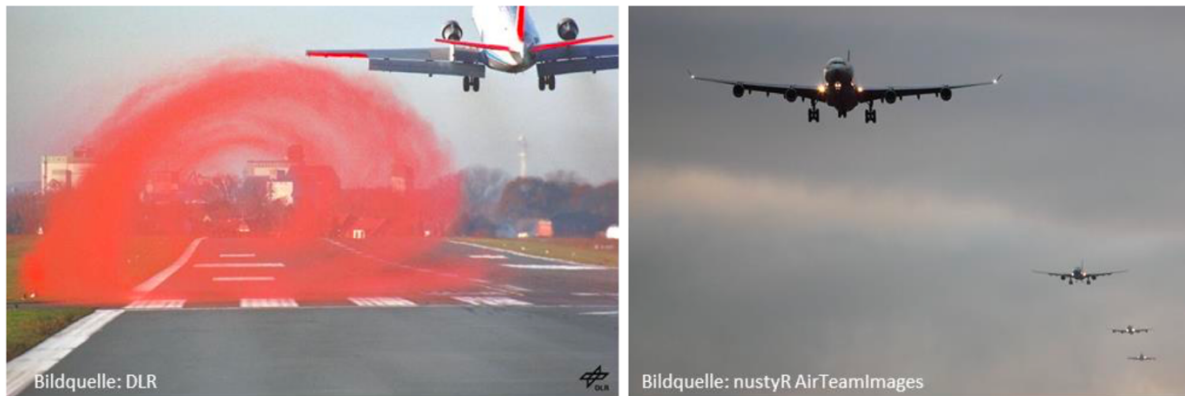
Figure 1: Visualization of the wake turbulence of the DLR research aircraft ATTAS (left); aircraft on final approach maintain a minimum distance from each other to avoid wake turbulence incursions (right).
