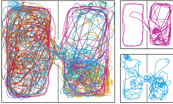
Figure 5: Trajectories of a resulting GP behavior traced for 10 minutes. Left: population of eight robots; right: two of the eight robots depicted separately.
