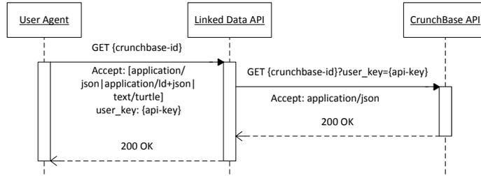
Fig. 2: UML sequence diagram illustrating the use of the wrapper. The wrapper supports different representations via content negotiation. The API key is passed to the wrapper via an `Authorization` header, and passed from the wrapper to the Crunchbase API as URI parameter.
