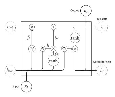
Figure 2.11.: Architecture of a recurrent cell in a Long Short-Term Memory Network (LSTM) with three different gating mechanisms  $\sigma_f$ ,  $\sigma_i$  and  $\sigma_o$  [Bia+17, p. 12].
