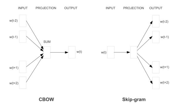
Figure 3.2.: FNN architecture of the Continuous Bag-of-Words (CBOW) and Skip-gram model [Mik+13]. CBOW uses context words to predict the target word. Skip-gram takes a word to model its context.
