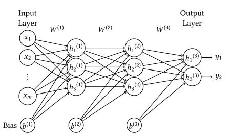
Figure 2.8.: Multilayer Perceptron with 2 hidden layers and 2 output neurons [Mar15, p. 72]. Three weight matrices connect the layers to pass the values through the network.
