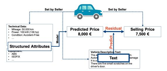
Figure 4.1.: A car has structured attributes, which are used to predict a market price. The seller of the car sets a price at which the car should be sold. The basic idea of my approach is the prediction of the price deviation between the predicted market price and the selling price by using the individual description text written by the seller. In this example, the price residual to be explained by a text is 500 €. (Car icon was retrieved from [Fla].)
