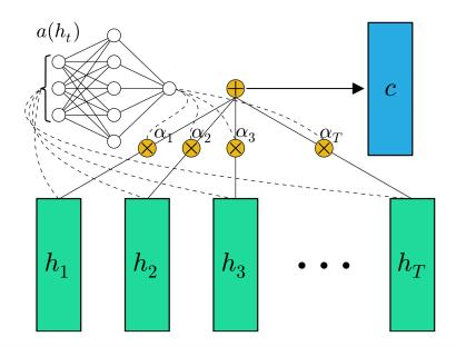
Figure 3.4.: Bahdanau Self-Attention applied to a RNN [RE15]. A FNN  $a(h_t)$  computes the attention weights  $a_1, \ldots, a_T$  to retrieve an averaged context state c.
