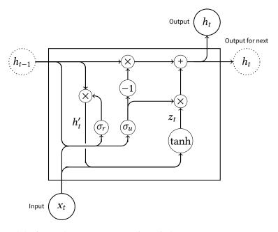
Figure 2.12.: Model of Gated Recurrent Unit (GRU) that uses two gates  $\sigma_r$  and  $\sigma_u$  to regulate the information flow within the network [Bia+17].
