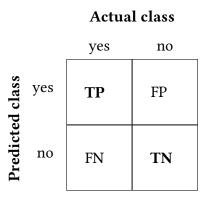
Figure 2.4.: Confusion Matrix contains the values for True Positives TP, True Negatives TN, False Positives FP and False Negatives FN. The matrix is illustrated for a binary class with two outcomes (yes, no).
